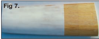
Fig 7. Apply paint primer once surface is flat and smooth. This tough, hard, resistant surface is now ready for painting.
