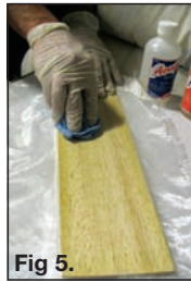
Fig 5. Lay glass cloth onto wet surface. Wet the cloth with more mixed resin. Remove excess resin with squeegee or cloth to give at this stage an almost dry appearance.
